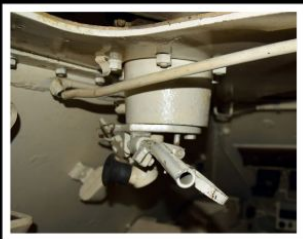
The tank's loader fired the roof-mounted machine gun by using the two handles to aim it at the target
